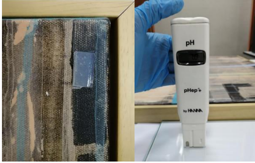
Image-13: pH measurement with agar agar method (Source: Serpil Çetinkaya 2022).
